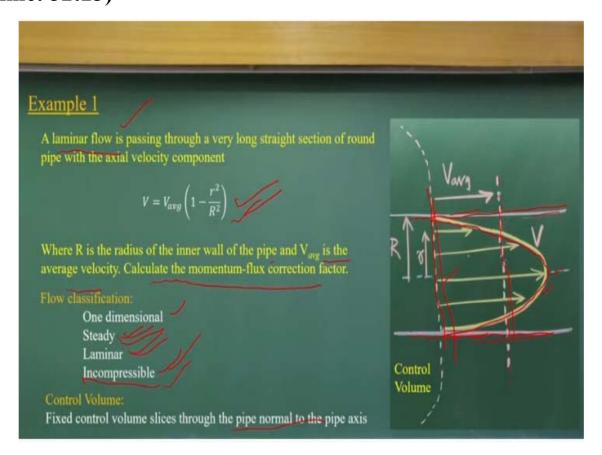
[A laminar flow is passing through a very long straight section of round pipe with the axial velocity component
