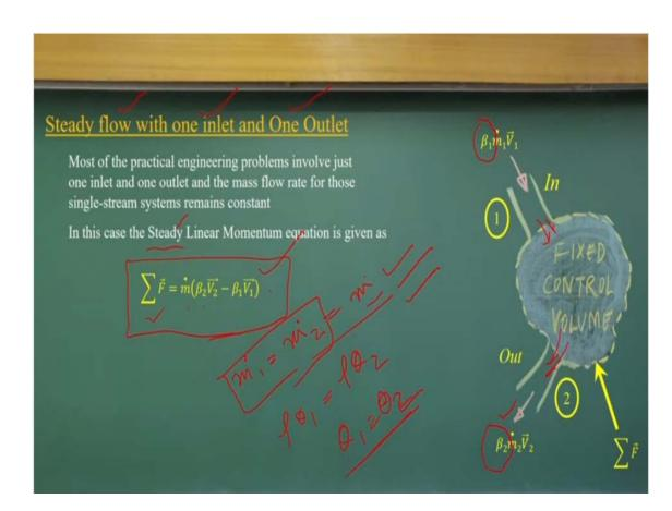
Now, let us go for another simplifications. That in a steady flow conditions, okay and only one outlet one inlet, this is very simplified case. See when you have one inlet and one outlet, if your mass influx is  $\dot{m}_1$  is inflow is coming into that, your mass influx out will be  $\dot{m}_2$ , that should be equal. That means,  $\rho Q_1 = \rho Q_2$  will be equal that means Q1 = Q2, that is a very basic equations what we get it, if we apply the conservations of mass.
