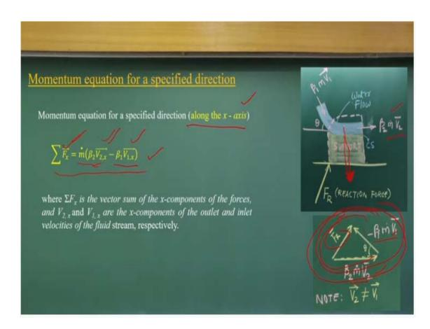
Now, there are the problems where is come it, very interestingly that we can apply the momentum equations as you can go it, this momentum equation is a vector equation, it has a three components in scalar directions, X component, Y component, Z component. Many of the time, we result at specific directions, in this case is X directions to find out the force components. That is what we try to look it, what will be the force is happening it, in the X directions only.
